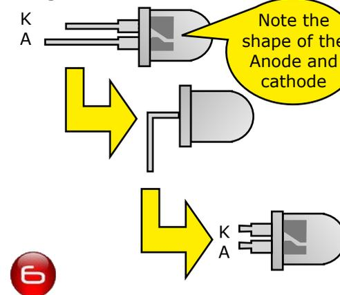
Now solder in place the prepared LED, ensure it is the correct way around. This can be verified by looking at the internal construction of the LED, see step 6.
