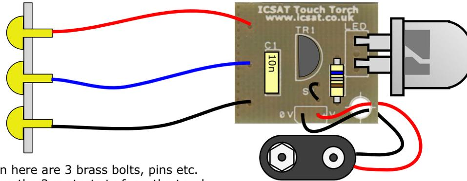
Shown here are 3 brass bolts, pins etc. Used as the 3 contacts to form the touch switch
