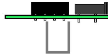
Solder it in place, so it connects the 3 switch pads together on the **underside** of the PCB
